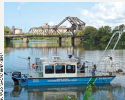
EPA Research Vessel Mudpuppy takes core samples to measure the extent of contamination in the sediment of the Buffalo River.
